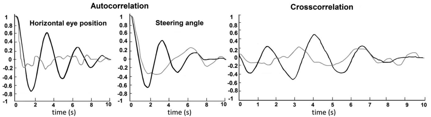
Fig. 1. Auto- and cross-correlation functions change with distraction. The grey lines represent the nondistracted condition and the black lines represent the distracted condition. The vertical axis is the correlation coefficient and the horizontal axis is the time lag.
