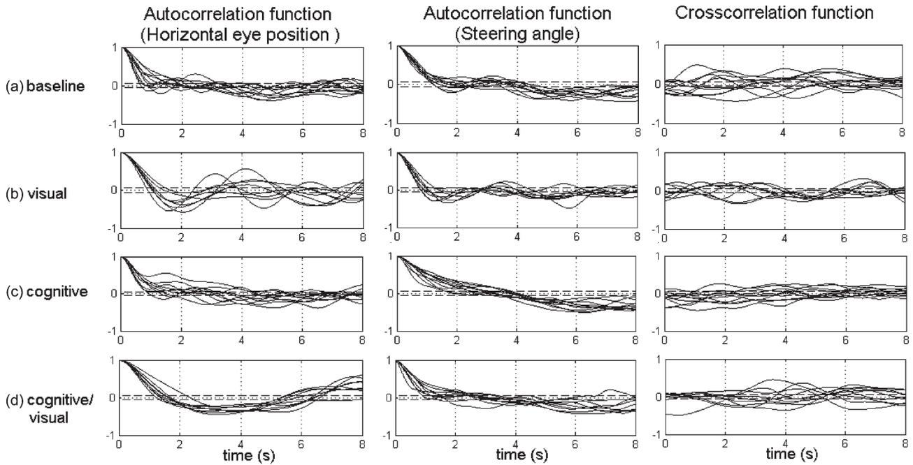
Fig. 3. Auto- and cross-correlation functions for detrended steering angle and horizontal eye position for nondistracted and distracted conditions. The functions were calculated for all the 30-s segments. The dashed lines are 95% CI.
