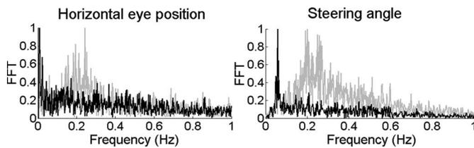
Fig. 2. (a) Steering angle and (b) horizontal eye position spectra for nondistracted (black line) and visually distracted (grey line) conditions.
